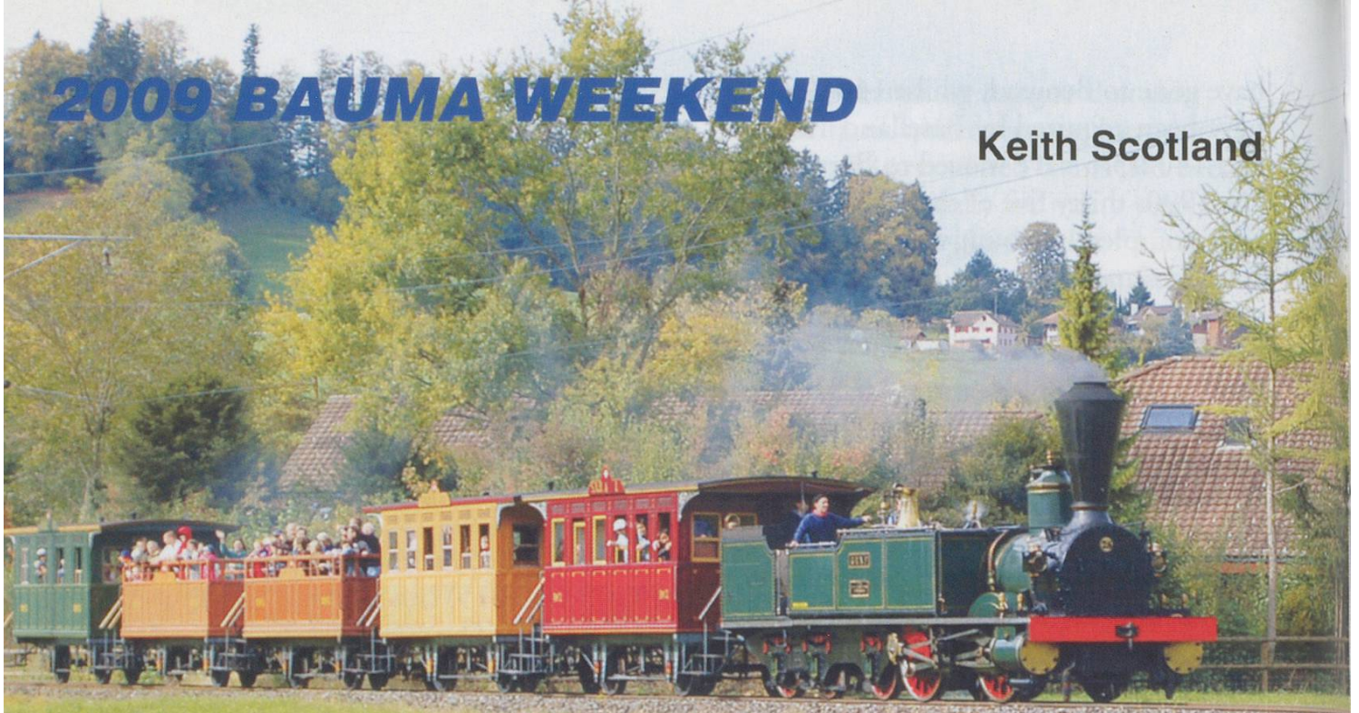
"Genf" Ec 2/5 of 1858, built by Kessler Esslingen, for the SCB, hauling the "Spanish Brottlbahn" set of coaches. ALL PHOTOS: Keith Scotland
