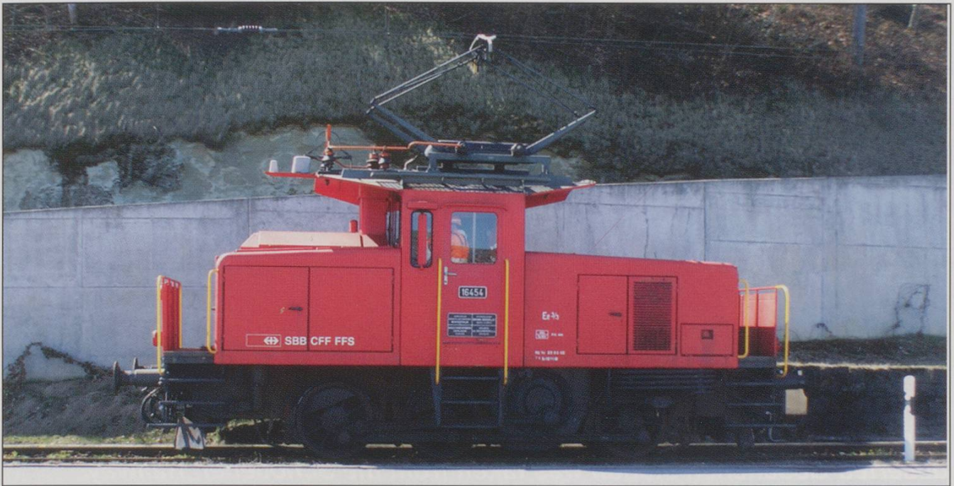
The works still justify a full-time Ee3/3 shunter seen here on the highway crossing outside the works...
