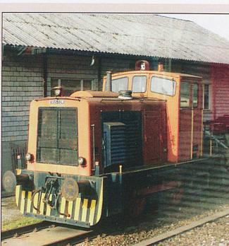
At Flüelen on a private siding (and not accessible) there is this four-wheel, side rod-transmission, diesel shunter built by Ruston in Britain. Bryan knows nothing of this engine, but it looks rather like those used on BR at one time, 11507 and 11508, built in 1956, of which his ABC tells him they had an 'SLM type friction clutch in a Ruston gearbox'. He wonders if its a cousin of those.
