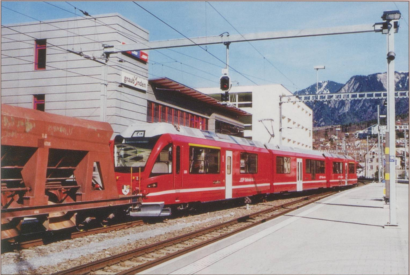
RhB Allegra ABe 8/12 No 3502 hauls a test train of hoppers at Chur.
