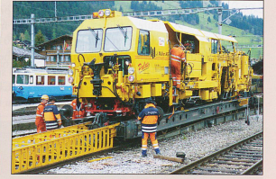
Unloading a track maintenance machine at Zweisimmen from the standard to meter gauge. PHOTO: Roy Marriott
