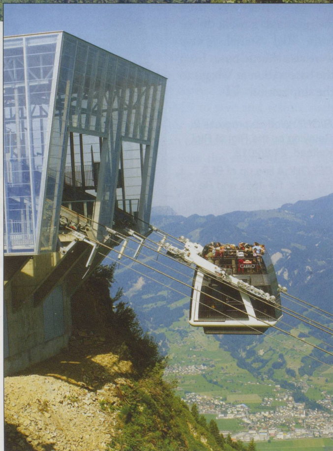
ABOVE: Seen from the upper deck of a parallel cable car, showing suspension from cables at its sides.
