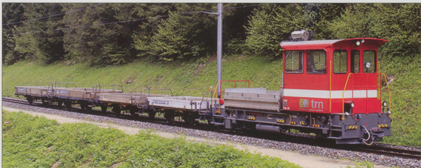
Bottom: TRNcmn Tm2/2 maintenance tractor.
