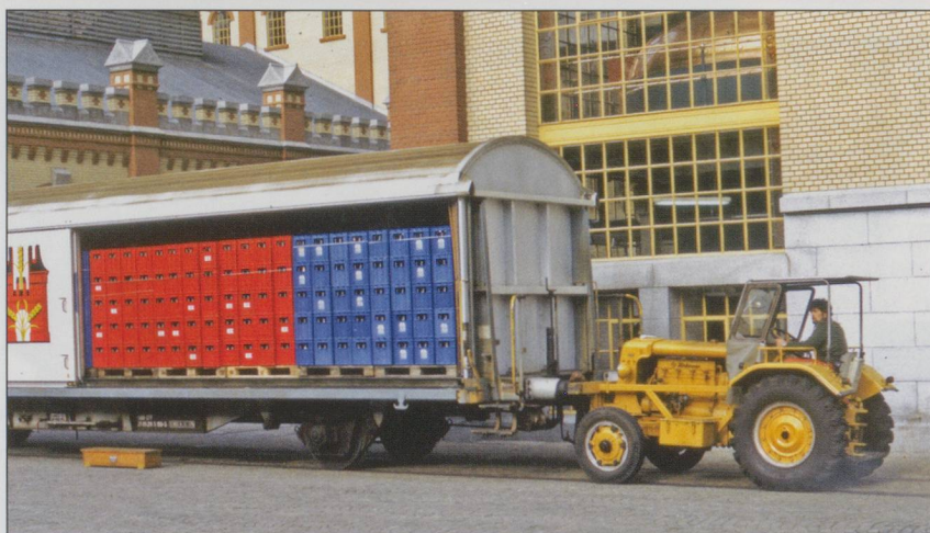
BELOW: A wagon being shunted by an adapted road tractor.
