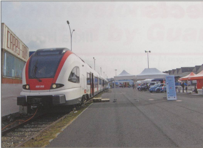
'FLIRT France unit open for the public view at Genève La Praille during a CEVA open day 26.9.2015. It has in addition to the standard 'Swiss FLIRT', support for the French 25 kV power and security systems: platform cameras, : French standard longer nose to absorb impact in case of a crash, and three types of power sockets for the passengers.
