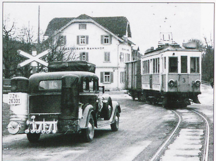
A car fitted with a 'Producer Gas' generator ,waits for UOe CFe 2/2 No.3 to leave Esslingen for Oetwil. 1946.
