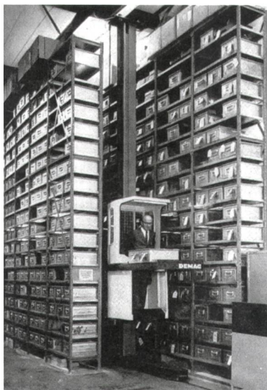
Fig. 14, A typical distribution center, interior view, showing a picker-crane and its driver, in: Joylon Drury / Peter Falconer, Building and Planning for Industrial Storage and Distribution , Oxford: Architectural Press, 2003, p. 171.
