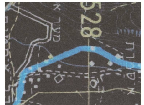
fig. d «The 0.02 mm border line at a 1:500 scale, Jericho» © Benjamin Leclair-Paquet
