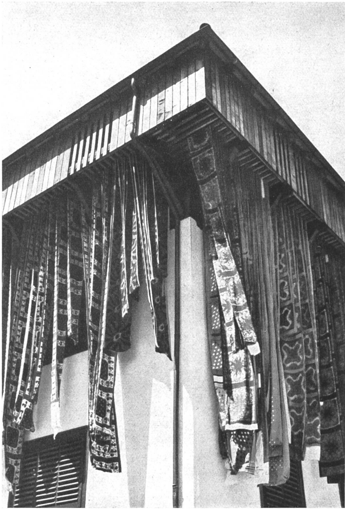
Even to-day printed fabrics can be seen drying in the open air, hanging from old «drying towers».
