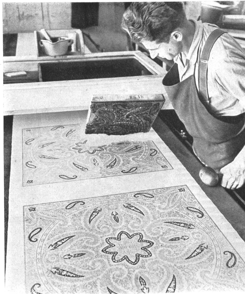
Printing by hand. The worker holds the mallet in his left hand. With the handle, he strikes the block to ensure perfect contact with the cloth.
