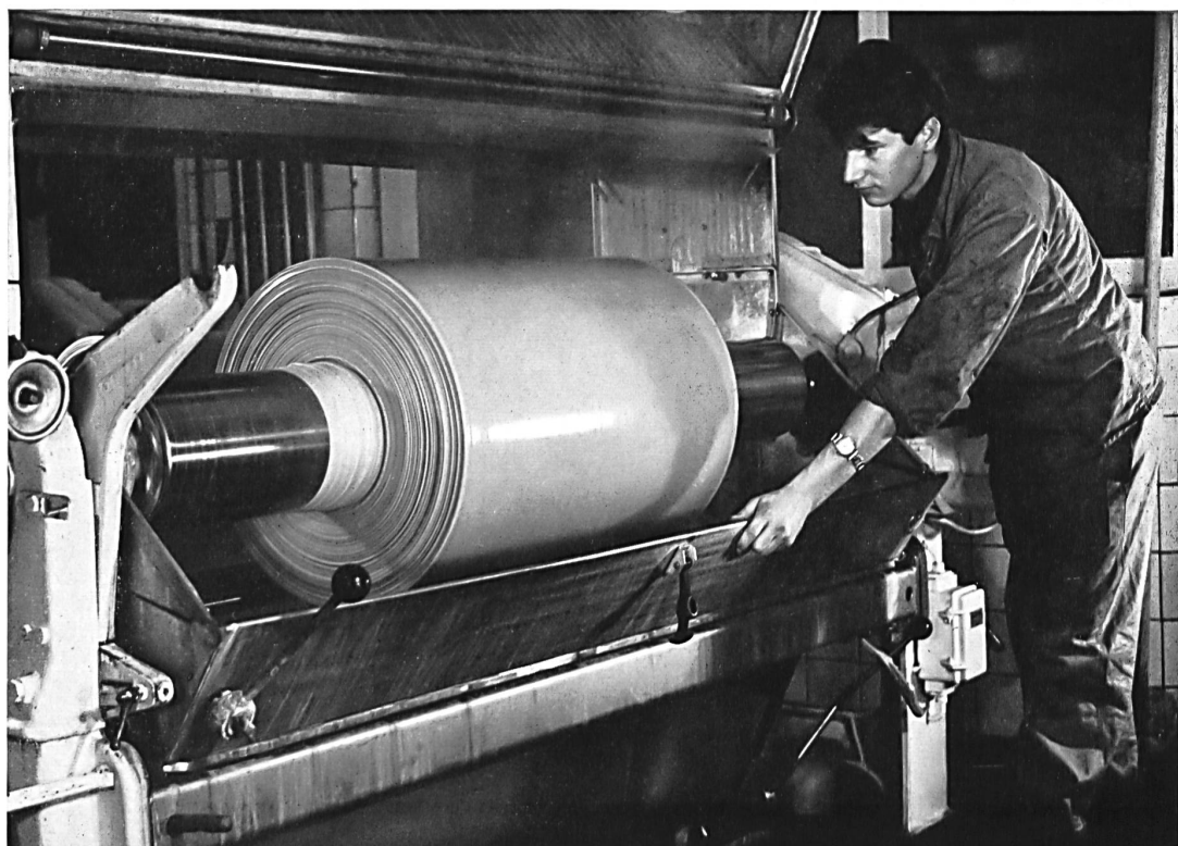
Piece dyeing on an automatic jigger
