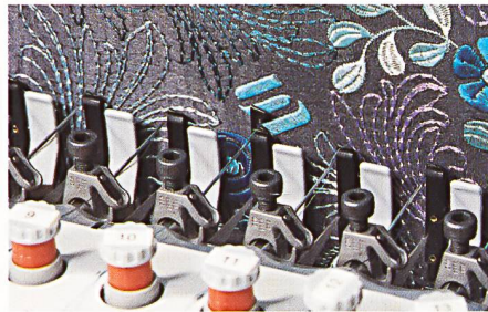
Pentacut thread cutting device on the needle side.
