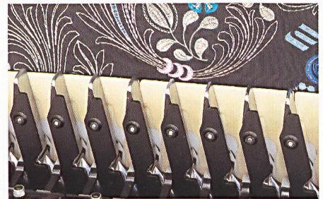
Pentacut thread cutting device on the shuttle side.
