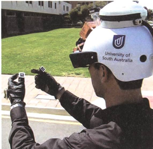
Tinmith Augmented Reality System from the University of South Australia, 2006
