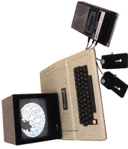
1977: Apple II, one of the first highly commercially successful personal computers, hit the market in 1977. It featured a colour display and came complete with two game paddles and a cassette interface for data storage. Photo: FozzTexx, Creative Commons
