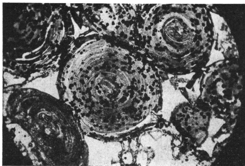
Fig. 2b. Thin section of oolitic chamosite with inclusions of magnetite \times 40 .
