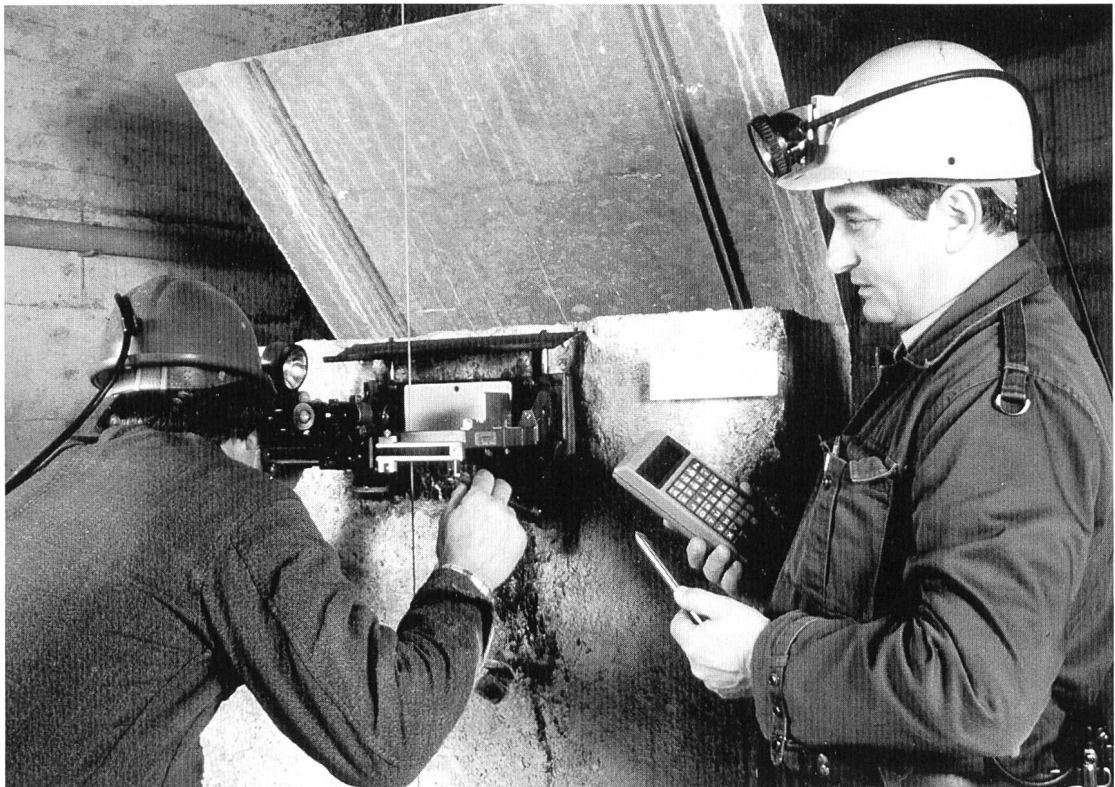
Figure 6.5. Automatic data gathering on a Palmtop pendulum in a dam inspection gallery.
