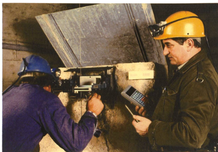
Figure 8. Measurement of pendulum deformation in a dam gallery. (Source: Emosson SA).
