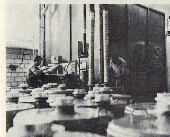
Test stand in our factory CH-8630 Muri, for the oil mist test and the resistance of gas filters.
